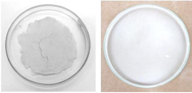
Figure 1. Phosphor ceramic adhesive coating cracking after 150°C (left) and water-based silicate paint binder coating with 10 airbrush-sprayed layers cured at 200°C (right).
